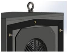
• Tighten the screws on the DHS cooling unit on the switch cabinet interior. Use the supplied screws, nuts and washers (accessory kit) to fasten the unit. Firmly tighten the screw fasteners to 12 ft-lbf (16Nm), or until seal is tightly squeezed.
